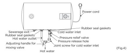
4. If the users want to realize a multi-way supply system, refer to the method shown in fig.5 for connection of the pipelines.
